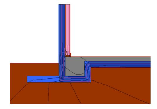
Thermally broken stem wall:  $\Psi = 0.018$  W/mK (0.010 Btu/hr ft F)
