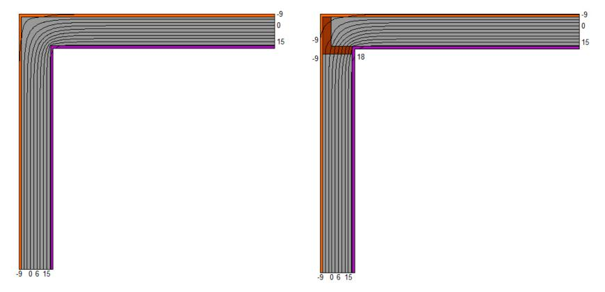
2x6 wall, no studs: Ψ = - 0.058 W/mK (-0.034 Btu/hr ft F) 2x6 wall, 2-stud: Ψ = - 0.040 W/mK (-0.023 Btu/hr ft F)
