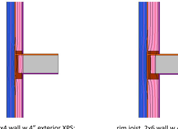
rim joist, 2x4 wall w 4" exterior XPS:  $\Psi = 0.011 \text{ W/mK}$ (0.006 Btu/hr ft F) rim joist, 2x6 wall w 4" exterior XPS:  $\Psi = ?$
