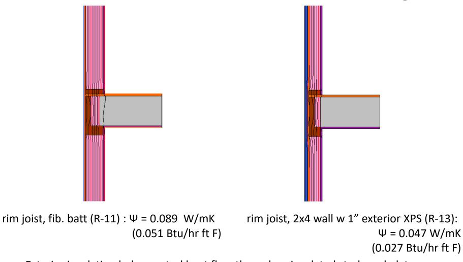
• Exterior insulation helps control heat flow through uninsulated studs and plates.
