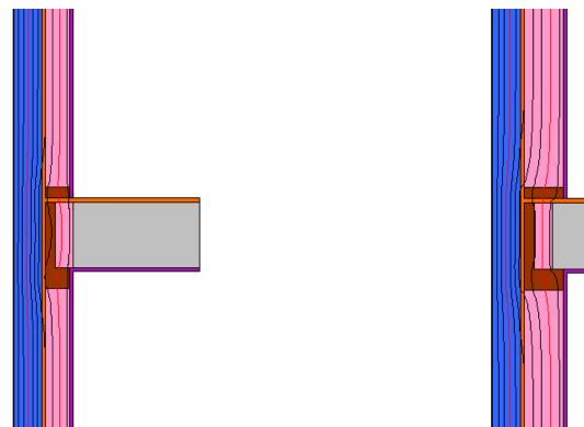
rim joist, 2x4 wall w 4" exterior XPS:  $\Psi = 0.011 \text{ W/mK}$ (0.006 Btu/hr ft F) rim joist, 2x6 wall w 4" exterior XPS:  $\Psi = 0.020 \text{ W/mK}$ (0.012 Btu/hr ft F)
