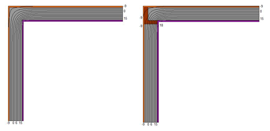
2x6 wall, no studs: Ψ = - 0.058 W/mK (-0.034 Btu/hr ft F) 2x6 wall, 2-stud: Ψ = - 0.040 W/mK (-0.023 Btu/hr ft F)
