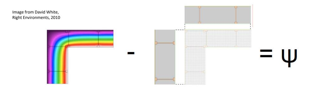
As used in the PHPP and WUFI Passive, the thermal bridge heat loss is conceptually the difference between the "true" heat loss, calculated using 2dimensional simulation (THERM or Flixo), and the heat loss calculated using the typical U<sup>-</sup>A method (U x A x deltaT = heat loss (or gain))
