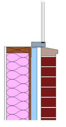
Window positioned outside of thermal envelope,  $\Psi = 0.10$  W/mK (0.058 Btu/hr ft F)
