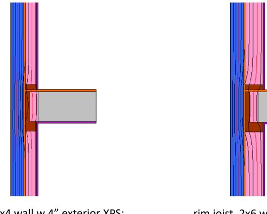
rim joist, 2x4 wall w 4" exterior XPS:  $\Psi = 0.011 \text{ W/mK}$ (0.006 Btu/hr ft F) Heat flux = 11.4 W/m rim joist, 2x6 wall w 4" exterior XPS:  $\Psi = 0.020 \text{ W/mK}$ (0.012 Btu/hr ft F) Heat flux = 9.9 W/m
