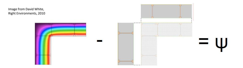
"2D heat loss" -  $U_1L_1 - U_2L_2 = \Psi$ L2d -  $U_1L_1 - U_2L_2 = \Psi$
