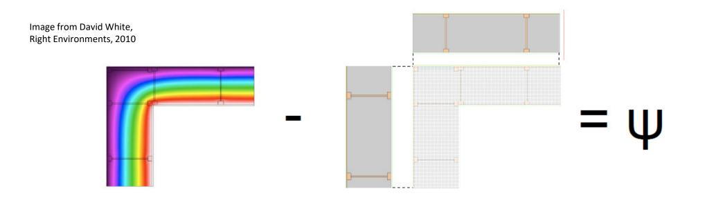
As used in the PHPP and WUFI Passive, the psi value is always based on a comparison of heat flows - a comparison between the actual heat flow and the estimated heat flow. In this sense, psi is a correction factor.
