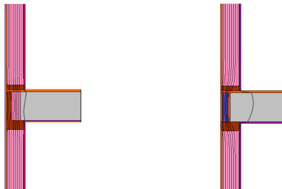
rim joist, fib. batt (R-11) :  $\Psi$  = 0.089 W/mK (0.051 Btu/hr ft F) rim joist, rim board (R-11):  $\Psi$  = 0.129 W/mK (0.075 Btu/hr ft F)
