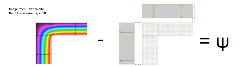
"2D heat loss"  $- U_1L_1 - U_2L_2 = \Psi$   $L2d - U_1L_1 - U_2L_2 = \Psi$  $\phi/\Delta T - U_1L_1 - U_2L_2 = \Psi$  (as in Flixo)
